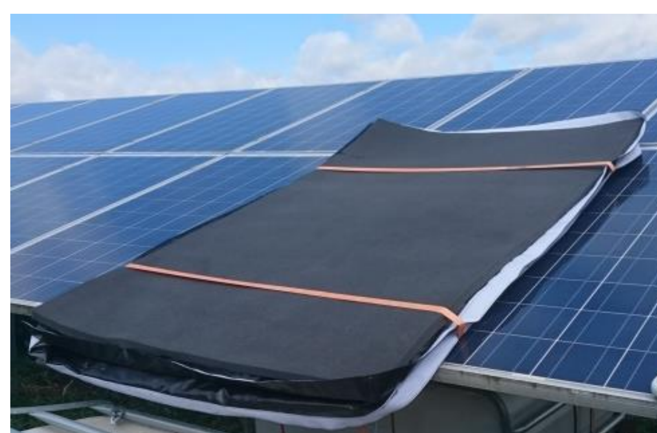
PID test with 'PIDcheck' prototype at remote location under harsh conditions (windy, rainy, cold)
