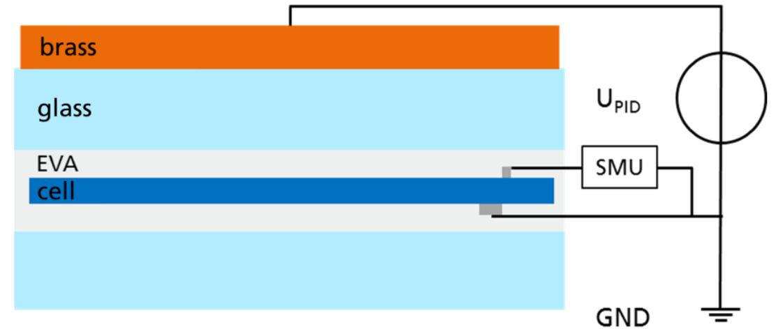
PID test set up: cell on ground level 0V, brass plate on high voltage  $U_{\text{PID}} = \pm 1000\text{ V}$ . SMU (Keithley 2601A) used for in situ dark-I-V
