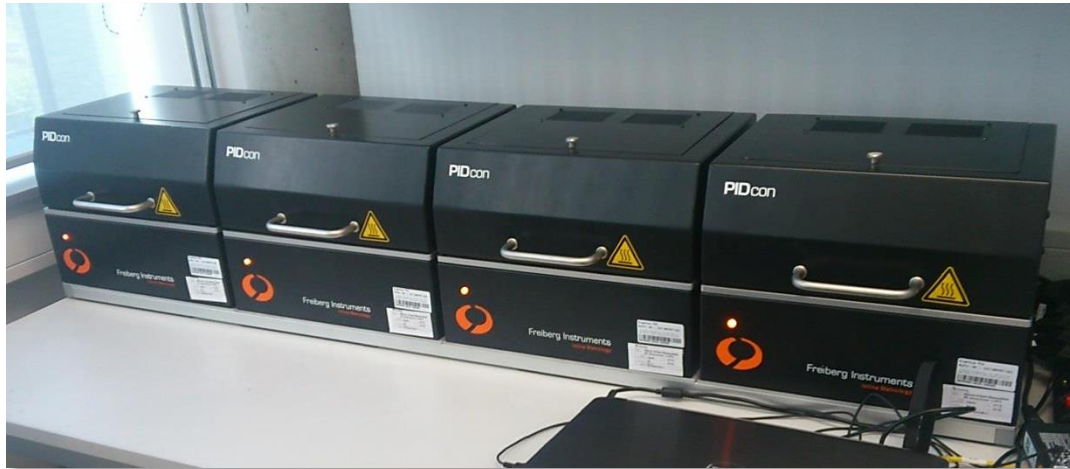
Four-fold PIDcon test device at Fraunhofer CSP
